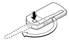
To retract the key, rotate it into the holder while pressing the release button.
